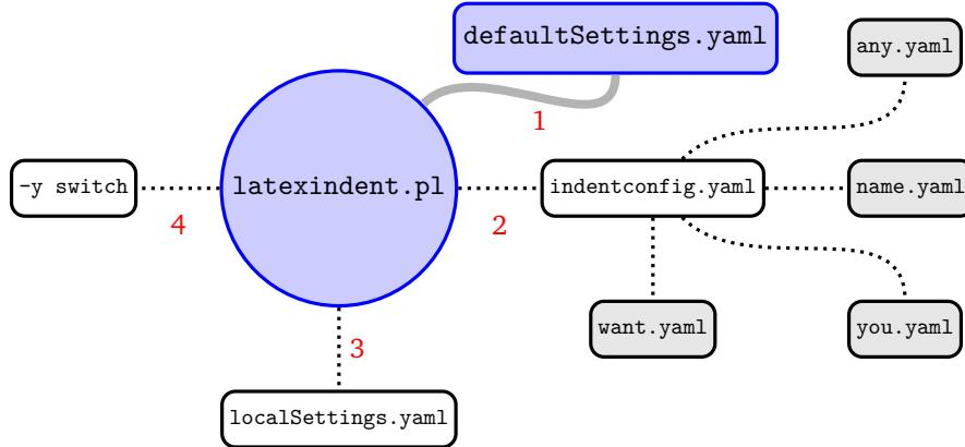
FIGURE 1: Schematic of the load order described in Section 4.4; solid lines represent mandatory files, dotted lines represent optional files. `indentconfig.yaml` can contain as many files as you like. The files will be loaded in order; if you specify settings for the same field in more than one file, the most recent takes priority.
